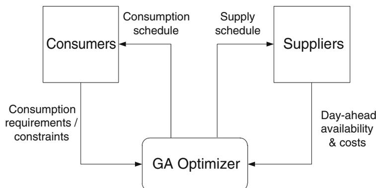
**Fig. 1** Flow of data in economic dispatch-DSM system. The suppliers will provide their day-ahead approximate availability and costs. The consumer smart home system will provide the system with consumption constraints. The
