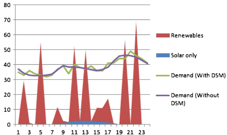
increase system efficiency. As an illustration of the outcome, Fig. 3 shows the total demand for 10 houses and the generation through wind and solar panels.
